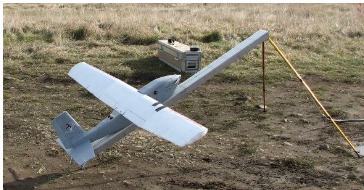
Photo taken in July 2012 in Christchurch, New Zealand under NSF RAPID grant support. Run-way independent take-off and landing; airline luggage transportability.
